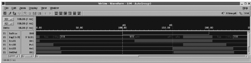
Fig. 14.9 Simulation of a delay line using enabled rnmos resistor models
